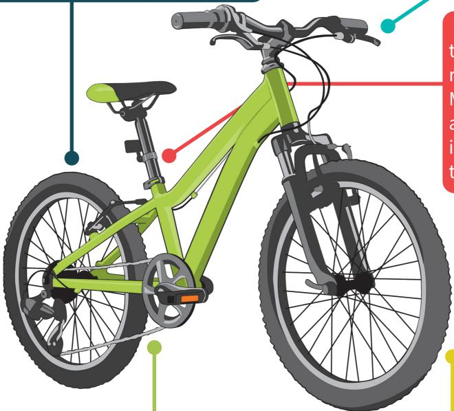
FIT – check that the seat post is not raised above the Min Insert marking as this can cause injuries and damage to the bike.
