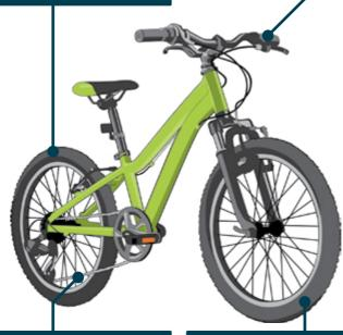
Chain – check the chain has clean oil on it and can move freely. The chain should look black or silver, not rusty. A little oil should come off if you touch it. If dirty oil has built up, clean that off first before adding more oil. Direction – with the front wheel "parked" between your legs, try to turn the handlebars firmly. The wheel should turn with the handlebars, and the handlebars shouldn't feel loose or wobbly.
